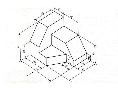
2. Draw to scale 1:1 the front view, top view and side view of the given machine block.
